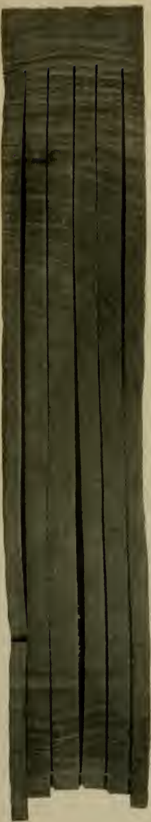
FIG. 24a.—Casehardening in a 2½-inch black walnut plank. This slotted disk cut from the plank clearly shows by the lengths of the prongs how great the internal stresses may become. Before slotting the prongs were all of the same length, about 14 inches.
