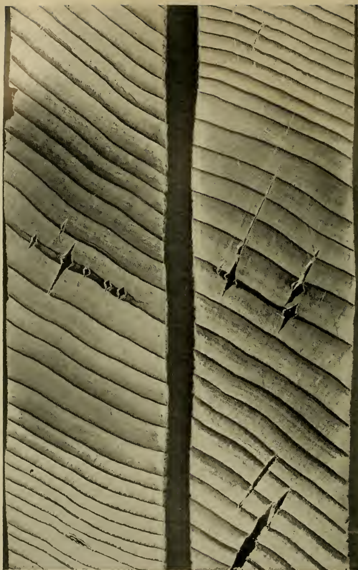
FIG. 43.—Magnified sections of western red cedar boards, showing the beginning of the "Explosive" effect.
